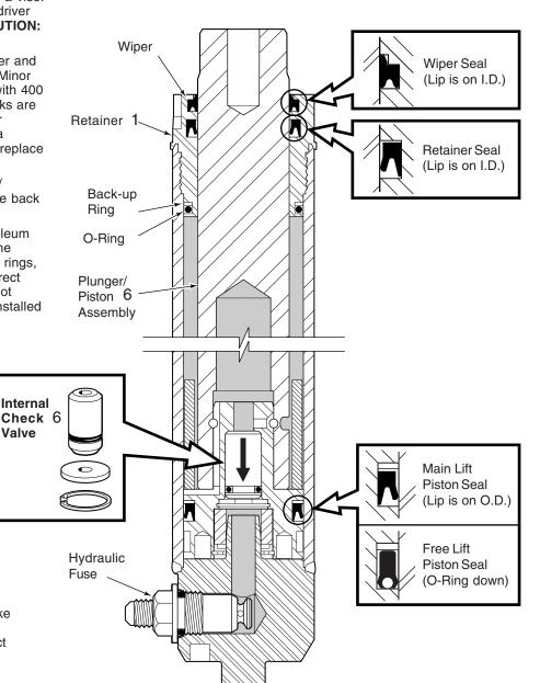
6 CYLINDERS WITH INTERNAL CHECK VALVE - When replacing the piston check valve O-ring, make sure the check valve is reinstalled with the arrow pointed in the correct direction.
